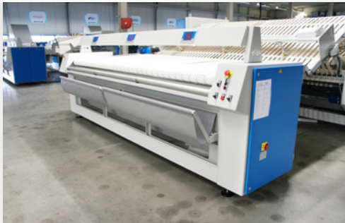
Control panel per lane to process different items
