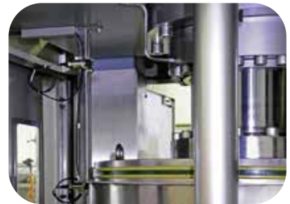
High-precision sensor technology for precise control of the ram position during pressing.
