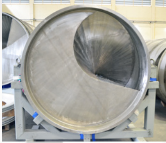
Large opening between compartments allows for reliable bottom transfer.
