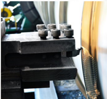
Flat-bar machining process for sealing.
