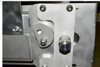
Easy to maintain tensioning device for pusher chain.
