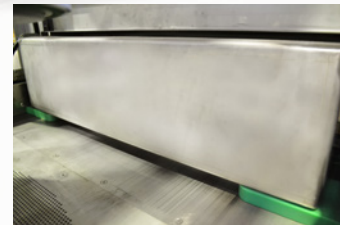
Stainless steel pusher providing a fast & efficient discharge of pressed batches.
