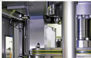
High-precision sensor technology for precise control of the ram position during pressing.
