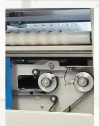
When pieces come out of the ironer they are measured by the photocell and counting-wheel on the feeding belts of the folder.
